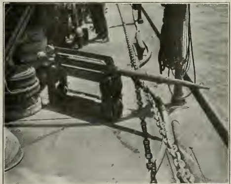
Jet nozzle. Cable passes through two sets of rollers below rollers. Lead weight is shown below rollers. (P. T. & T. Photo.)
